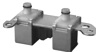
T76420 AODE/ 4R70W Shift Pack Fits 92-97 AODE, 95-97 4R70W 20-40 Ohms per solenoid, OEM Plug Compatible
