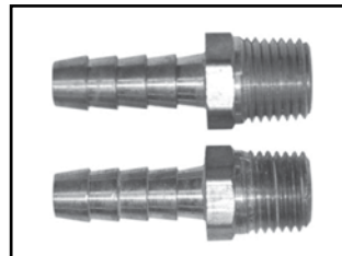
CR-1003 3/8" Hose Barb to Male 1/4" Pipe NPT CR-1004 5/16" Hose Barb to Male 1/4" Pipe NPT
